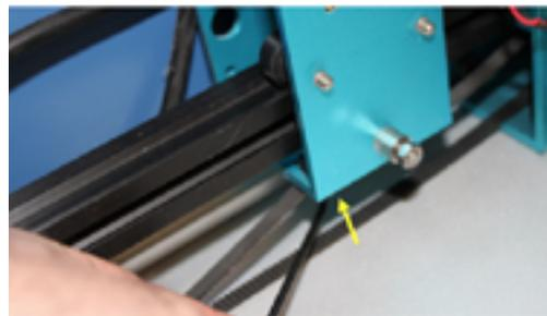
5. Loosen the idler pulley mount
