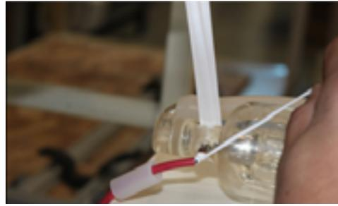
6. Bring the opposite side of the Teflon tape around the neck of the laser tube and around the inside of the electrode.
