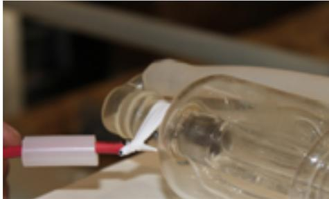
10. Fill the silicone tubing with silicone sealant.
